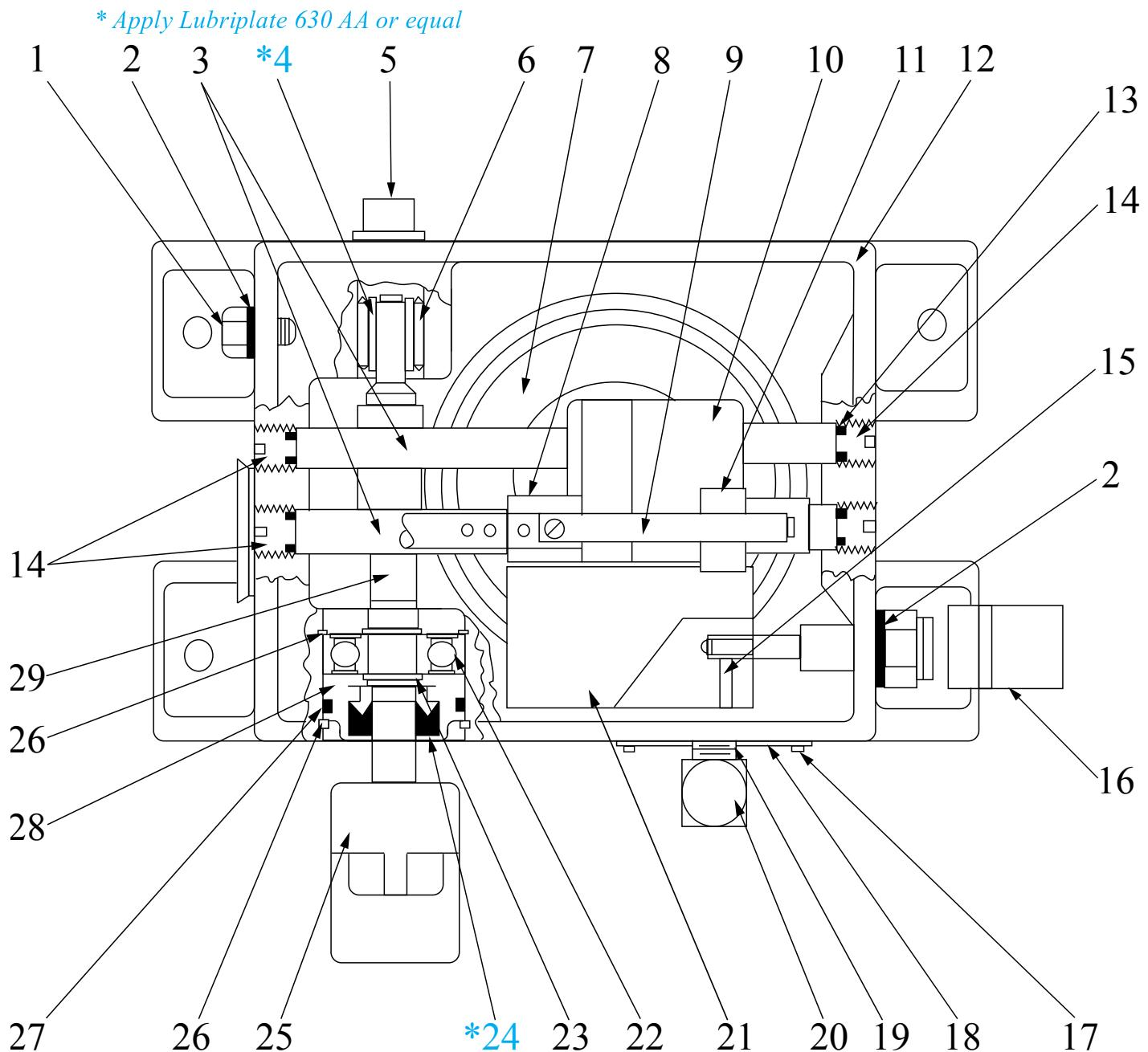
\* Apply Lubriplate 630 AA or equal between shaft and seal lips
